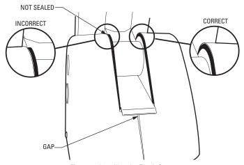
Figure 4. Installing the Esprit Cover
